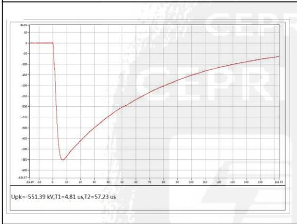
The 1<sup>st</sup> negative impulse waveform
